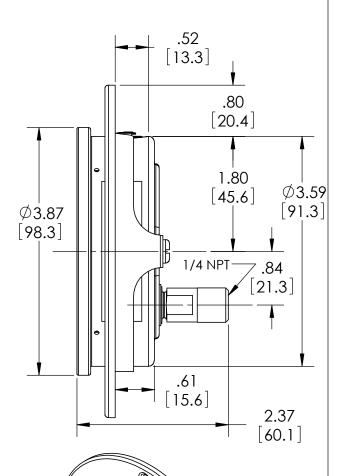
NOTE 1: PANEL CUTOUT- Ø3.78[96]MIN, Ø3.86[98] MAX NOTE 2: PANEL THICKNESS- 1/16[2] TO 1/4[6]
