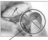
**CAUTION:** Diaphragm is fragile. **DO NOT PUSH ON IT** to test pointer response!
